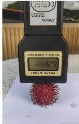
Figure 2. Quasi-static compression test by Force Gauge
